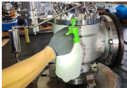
Valves: leak test
